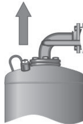
Eyebolt at vessel
